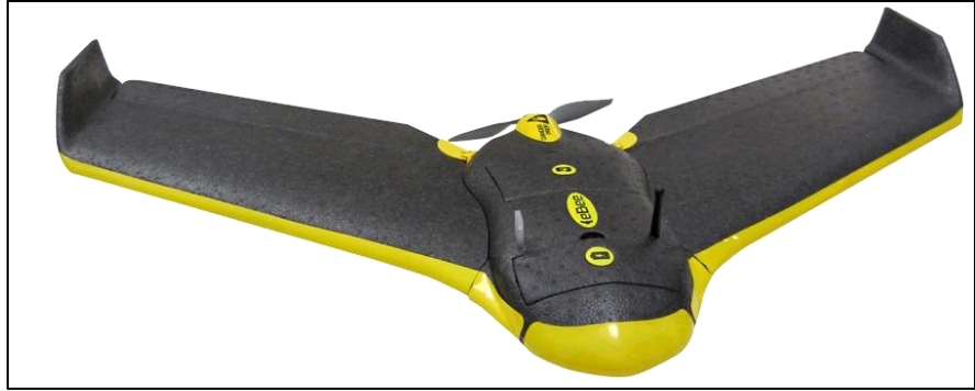
Figure 10: UAV used to collect high quality topographic data.
