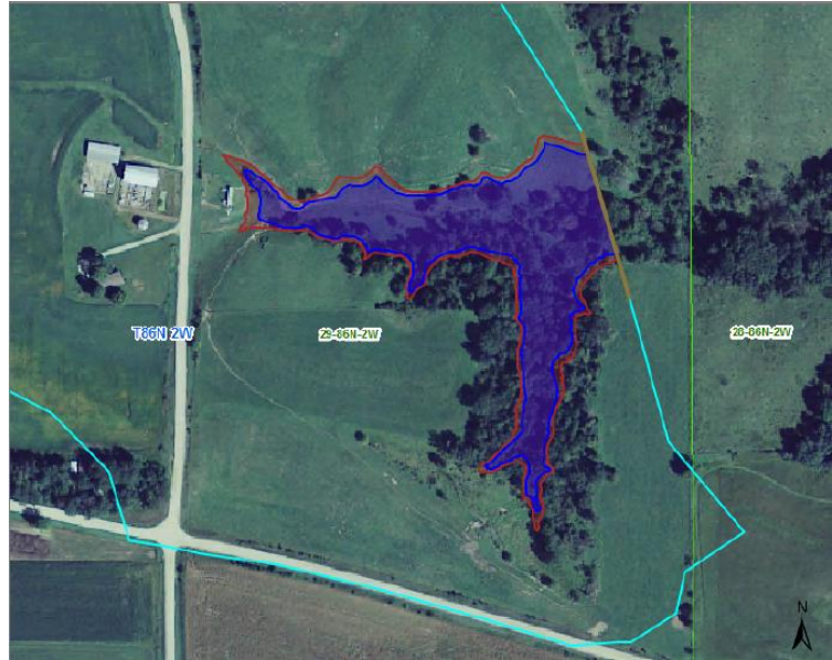
Figure 2: Pond design generated by Agren® PondBuilder.
